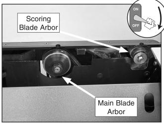
Figure 29. Main blade arbor components.
